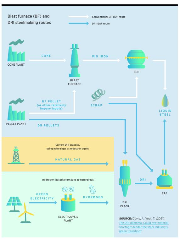
DRI is typically used in electric arc furnaces (EAFs), while blast furnace pig iron is consumed in basic oxygen furnaces (BOFs).
